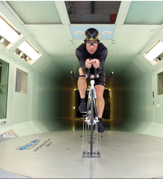
Tour de France champion Lance Armstrong testing a bicycle at the San Diego Air & Space Technology Low Speed Wind Tunnel in November 2008. Armstrong's clothing, helmet, posture, and hand position are also aerodynamically optimized.
