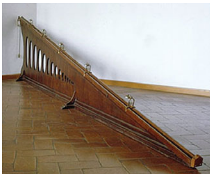
FIGURE 9 Apparatus of the type used by Galileo to study the motion of falling objects.
